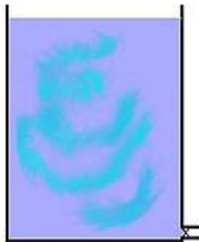
4. Permit the tank to stand for 24 hours if possible, but for no less than 6 hours
